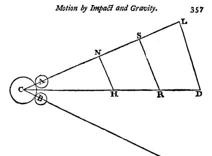
city of c after the stroke be represented by x, and that of A or B in the direction Ac or cB by y, and suppose p:q:: rad.: cosin. LcD. Then, because ma the quantity of motion before the stroke is equal to  $mx + \frac{2qny}{p}$ , the quantity of motion after the stroke, and  $ma^2$  is equal to  $mx^2 + 2ny^2$ , because the quantity of force is not altered by the collision; he easily finds  $x = \frac{p^2ma - 2q^2na}{p^2m + 2q^2n}$  and  $y = \frac{2pqma}{a^2m + a^2n^2}$ .
